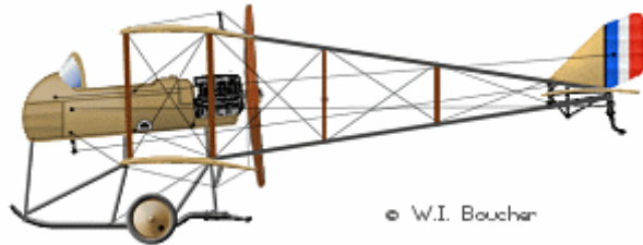
A Maurice Farman training plane of 1914. It was fitted with a radial Gnome engine and "pusher" airscrew
